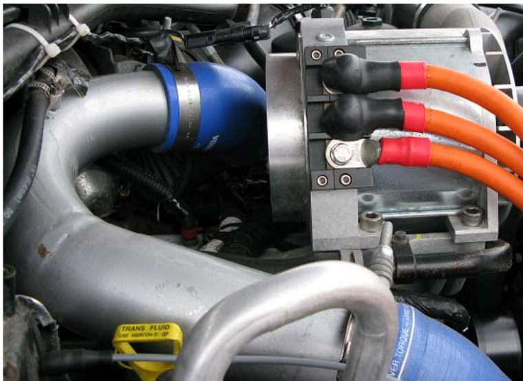
Powergain Alternator and Turbo Piping Rerouting
